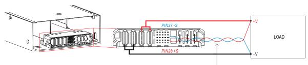
Sense lines should be twisted in pairs to minimize noise pick-up.
